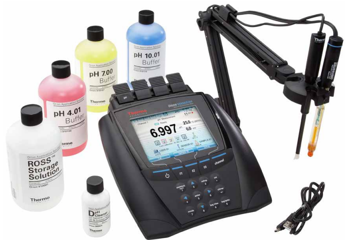
Thermo Scientific Orion Star A2114 Meter Kit (Cat. No. STARA2114) including calibration standards and ROSS Sure-Flow pH Electrode.
